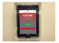
Have the students sign-in by reading a barcode with the iPad's front camera while keeping the device locked to display a classroom's scheduled courses through out the day in a tamper-free kiosk mode.
